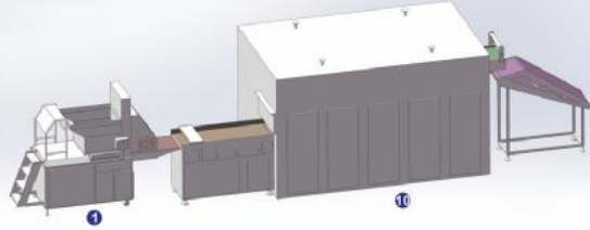
Automatic burger (beef, chicken, fish) and potato patty processing line
